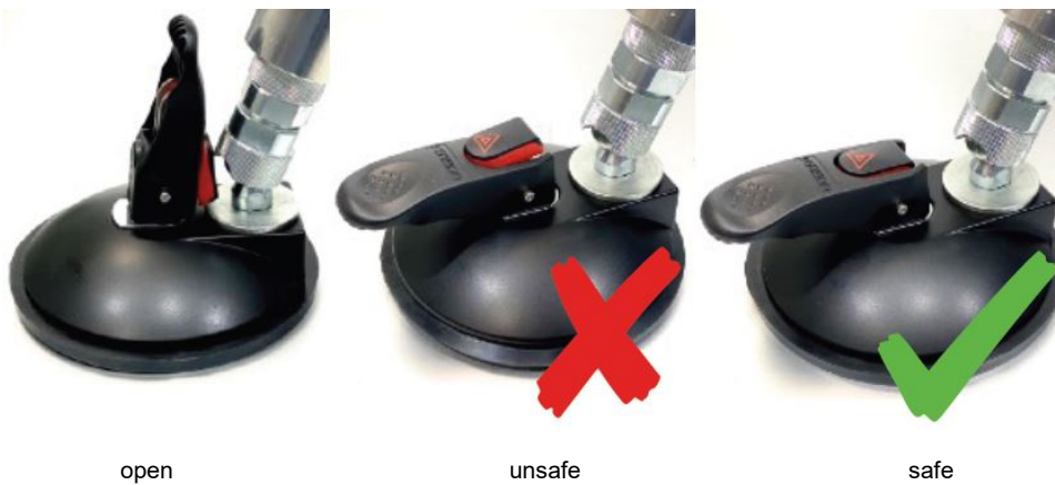
Suction cups with indicator Figure 17
